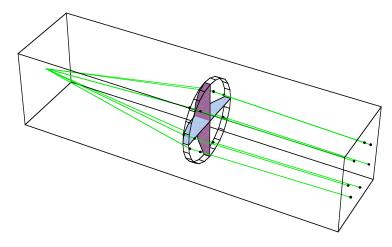
Note that this time, in order to position the **PlanoConvexLens**, we have passed the single numeric parameter of 100 to the **Move** function. When only single number is given to **Move**, the **PlanoConvexLens** is simply displaced along the x-axis by the given amount.
