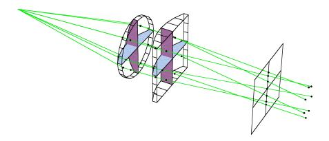
By using PlotType->Surface with RayChoice->{ComponentNumber->3}, you can clearly see ray intersection points at the screen surface.
