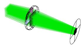
$\label{eq:analyzeSystem} $$\operatorname{GaussianBeam}[10, 0.1, \operatorname{FullForm} \to \operatorname{True}, \operatorname{NumberOfRays} \to 11],$$\operatorname{Move}[\operatorname{PlanoConvexLens}[100, 50, 10], 50.], \operatorname{Move}[\operatorname{Screen}[50], 150.]\}]$$
