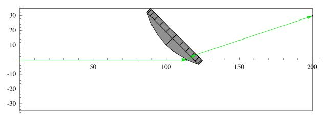
Here the rendered result shows three arrows that correspond with the three ray segments previously calculated by Analyze: System during the trace. ShowSystem and AnalyzeSystem both use the same options for graphical rendering. Although there are a great many options available for graphical rendering, some of most important options are listed in the following table.
