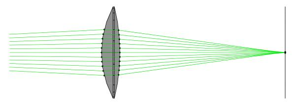
As one final speed-up, we can add the option **SequentialTrace** -> **True** to **OptimizeSystem**. Both **OptimizeSystem** and **TurboTrace** use **SequentialTrace** -> **False** by default. In this case, however, we can use **SequentialTrace** -> **True** because the rays in this optical system are all passing through the same sequence of optical surfaces without back-tracking or having multiple bounces.
